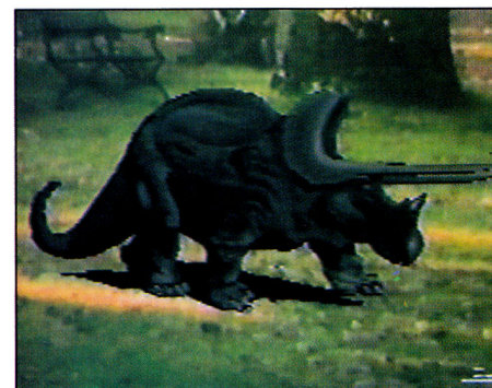
Overlay Card mixes computer graphics and video signals; here, DeluxePaint clip art overlaid on video frame.
